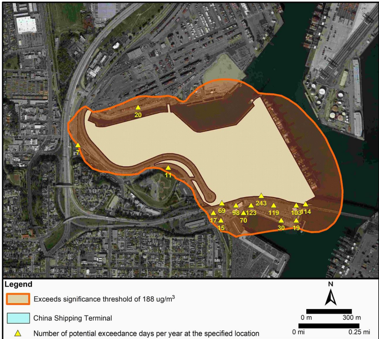
7 Figure 3.1-4. Area of Threshold Exceedance for the Revised Project; 2014 Federal 1-Hour 8 NO 2 Concentrations
