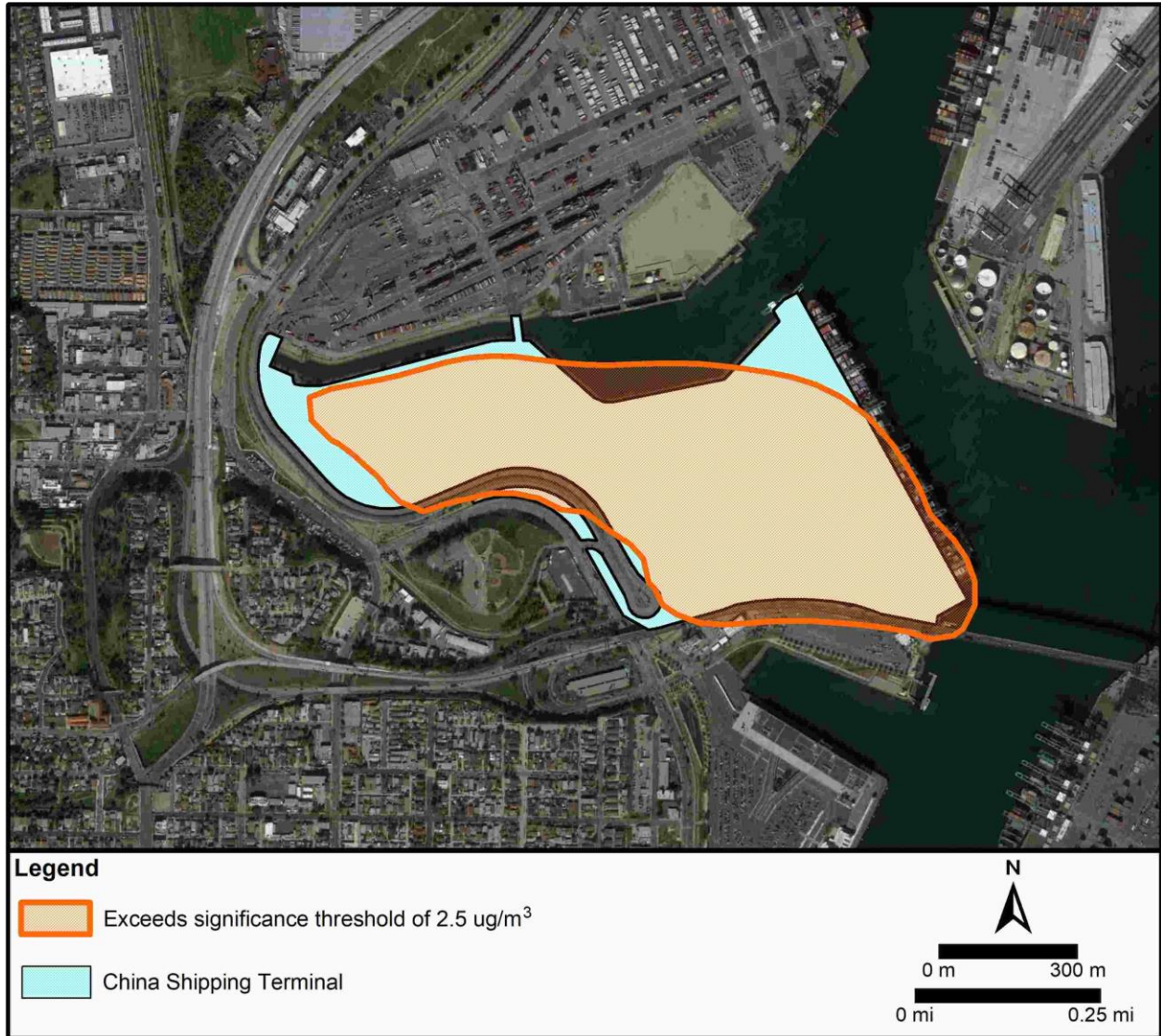
Figure B2-17. Area of Threshold Exceedance for the Revised Project; 2036 24-Hour PM 10 Concentration Increments
