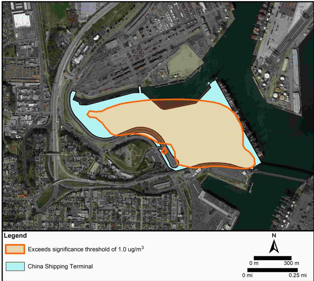
Figure B2-33. Area of Threshold Exceedance for the FEIR Mitigated Scenario; 2023 Annual PM 10 Concentration Increments
