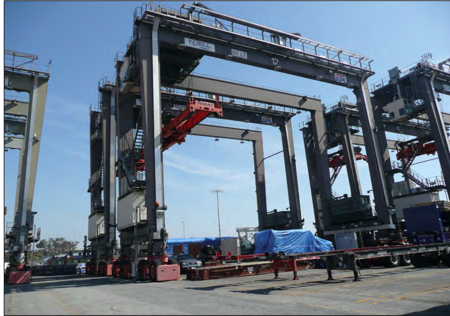
Photograph 12: Rubber Tire Gantry Crane
