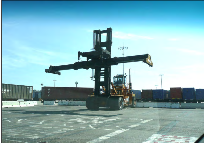
Photograph 14: Top pick or handler
