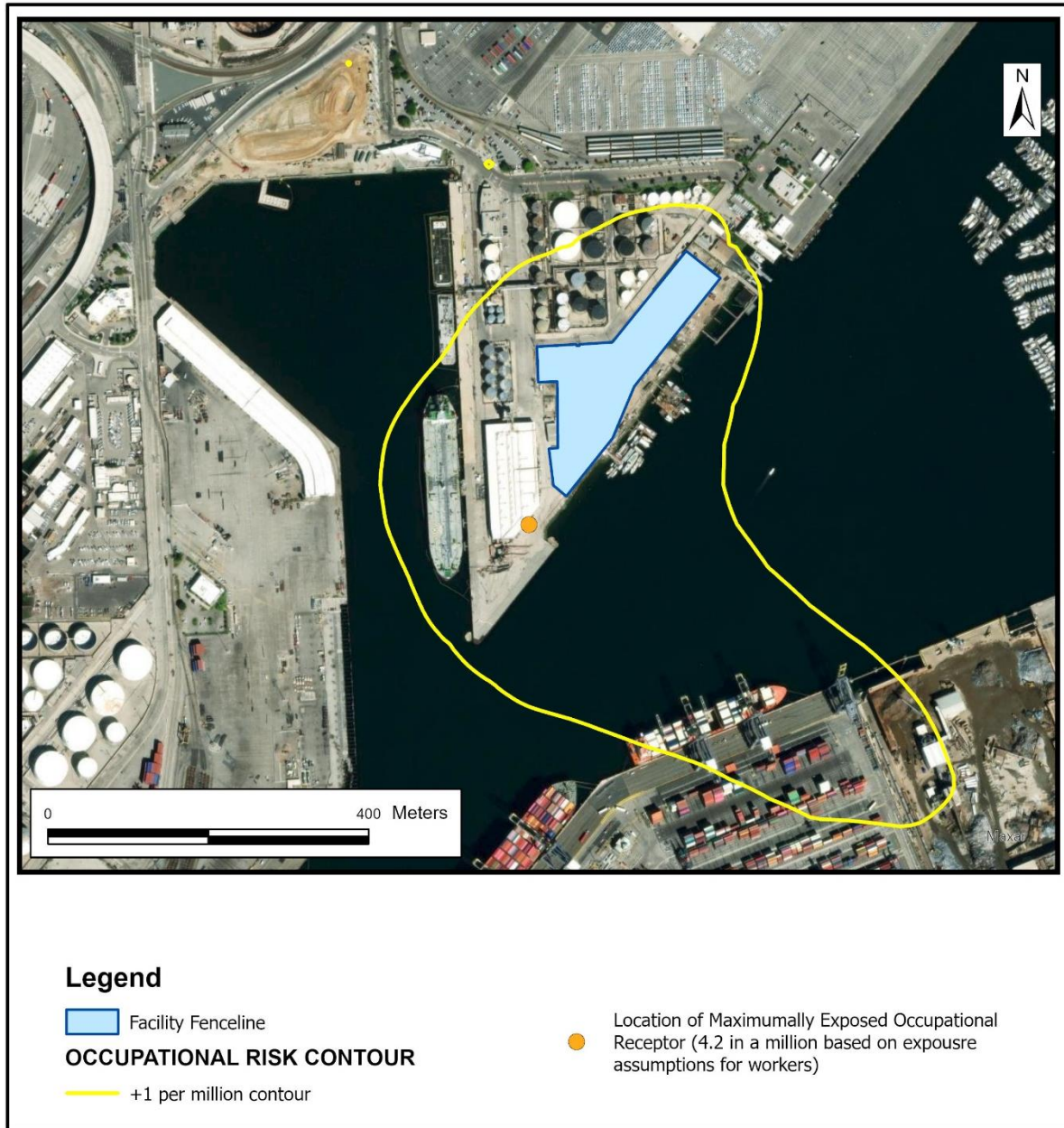
1 Figure 3.1-7 Isopleth of 25-year Occupational Cancer Risk – Product Import Terminal 2 Alternative (Alternative 3)
