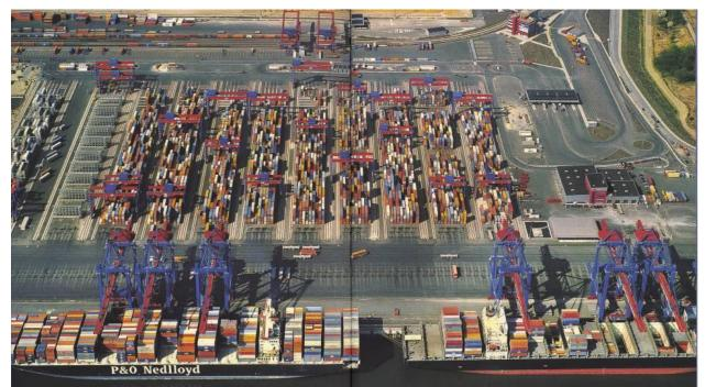
Figure A.3 CTA Hamburg's ASC+AGV operation
