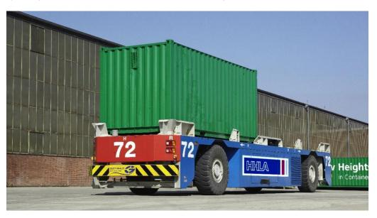
Figure A.2 AGV APL proposes to use unmanned rail mounted gantry cranes (RMGs) also known as automated stacking cranes (ASCs) to stack the containers. AECOM is aware of three other AGV+ASC type automated terminals in the world:
