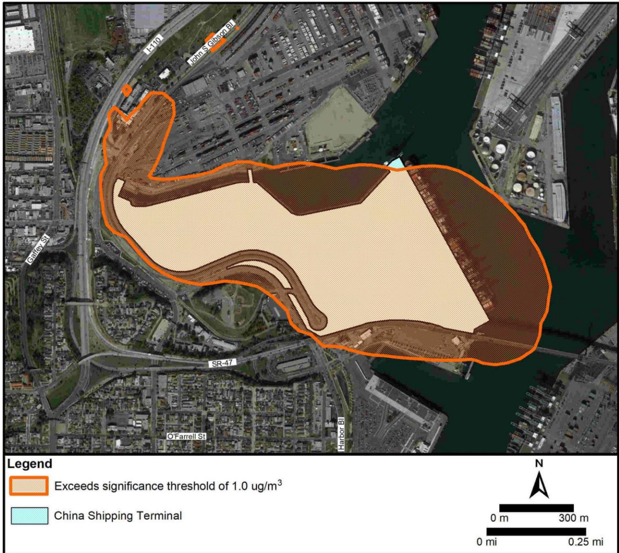
Figure B2-36. Area of Threshold Exceedance for the Revised Project; 2022 Annual PM 10 Concentration Increments
