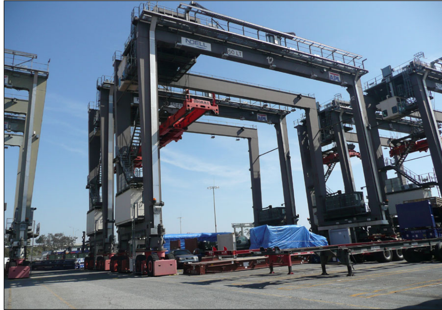
Photograph 12: Rubber Tire Gantry Crane
