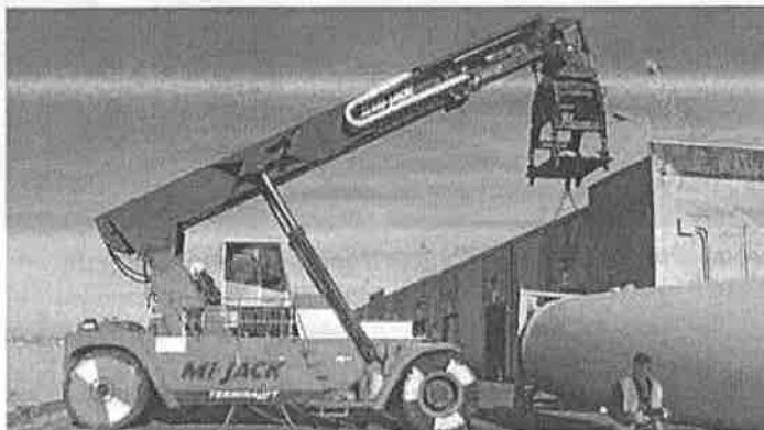
Figure 9. Electric reach stacker in operation.
