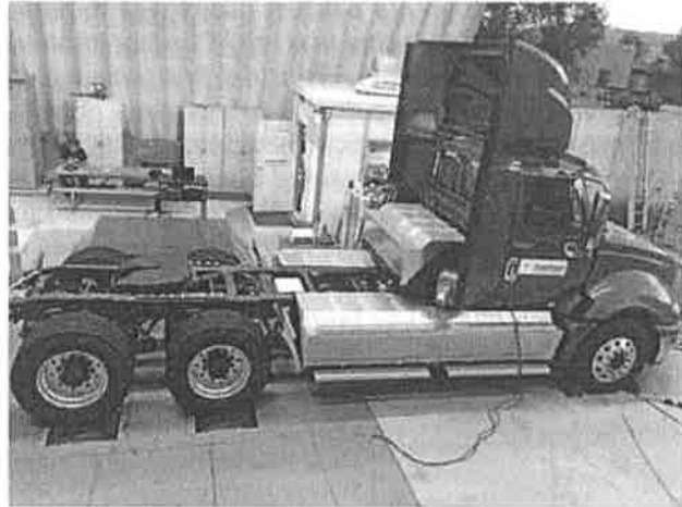
Figure 4. Latest EDD truck to enter service, during dynamometer testing in October 2014.
